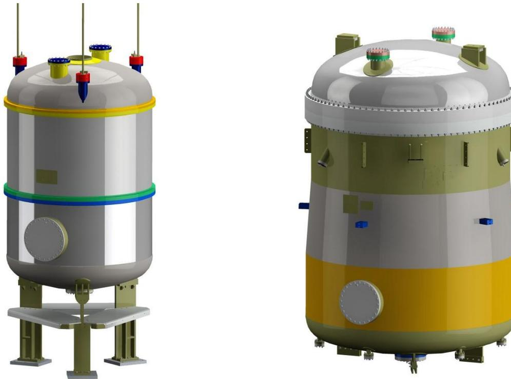
(a) The outer cryostat vessel and cryostat support.
