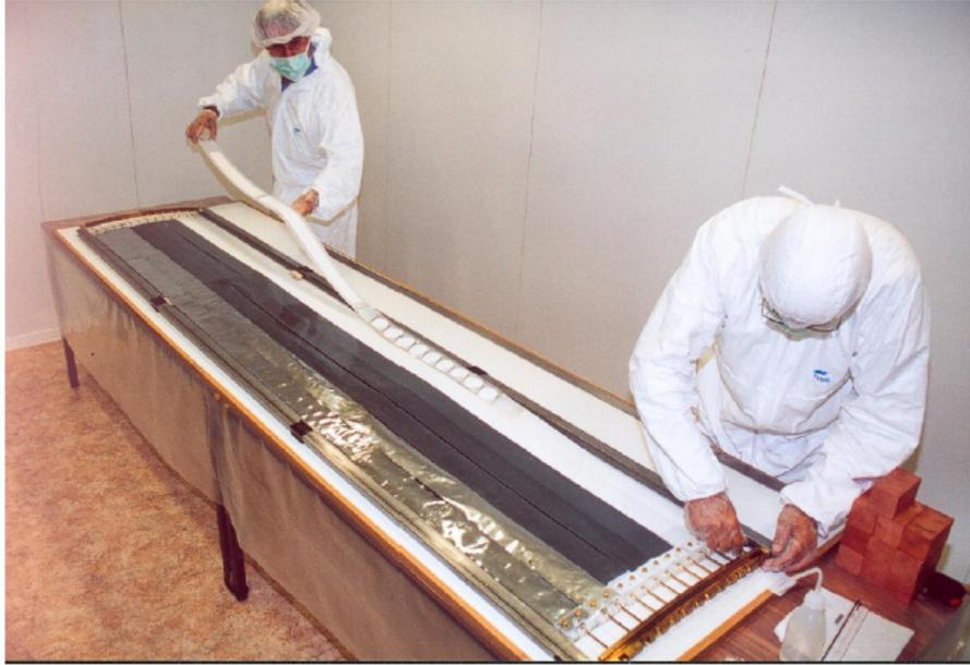
Figure 4.5: Preparation of sector 5 source which contains Ca discs. [147]
