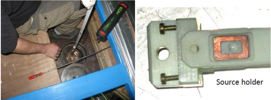
Figure 8.5: NEMO3 manual source delivery system and holder.
