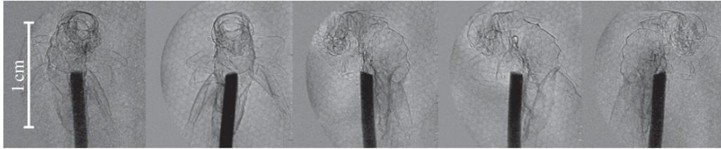
**Figure 1.6.:** Phase contrast image of a cricket taken with the Astra Gemini betatron source. Images show minimal absorption, indicative of high flux of photons at energies greater than 20 keV, for which the phase-shift cross section greatly exceeds that of absorption by more than 100 times [6].
