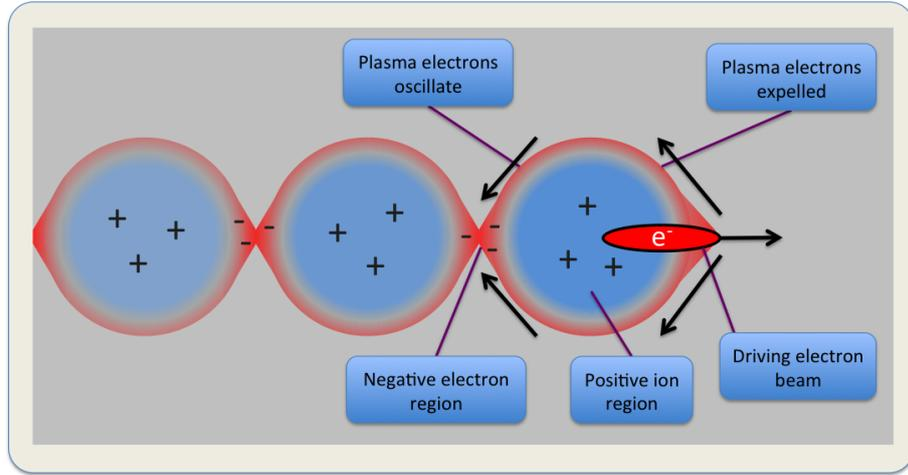
**Figure 1.3.:** A graphic of a short relativistic electron beam driving a plasma wakefield. The perturbed plasma electrons form a wakefield that co-propagates with the driving beam. An electron between an electron region and ion region will experience a strong longitudinal electric field.
