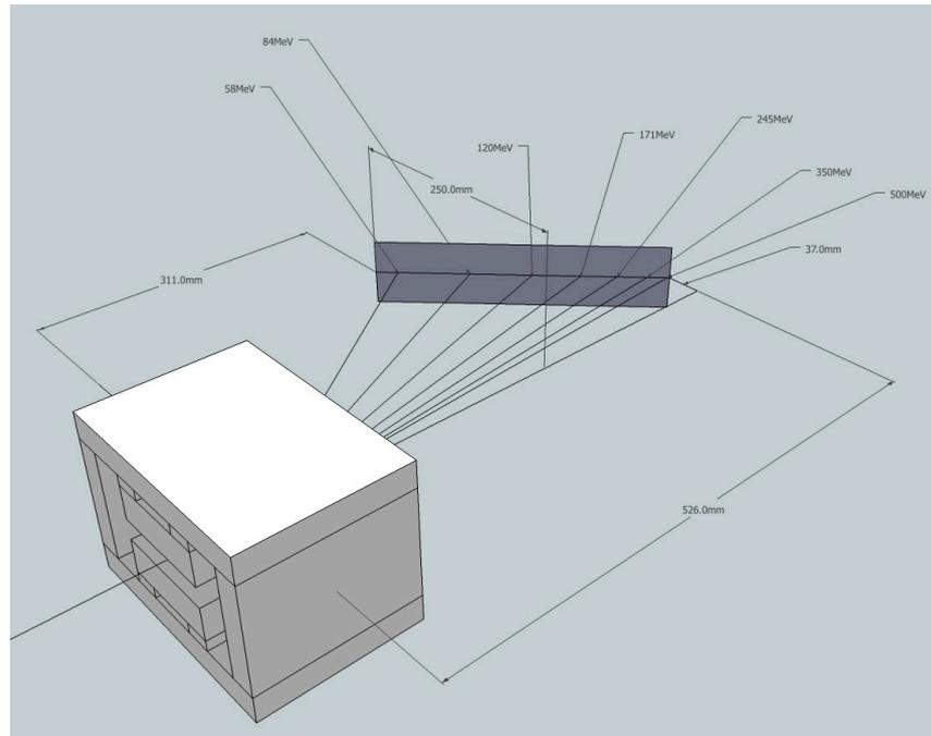
**Figure 6.6.:** Schematic of the electron spectrometer used in the TA2 experiment. A  $B = 1$  T magnet bends the electrons according to their energy onto a lanex screen where the spectra are recorded by a camera positioned behind the screen (not shown).
