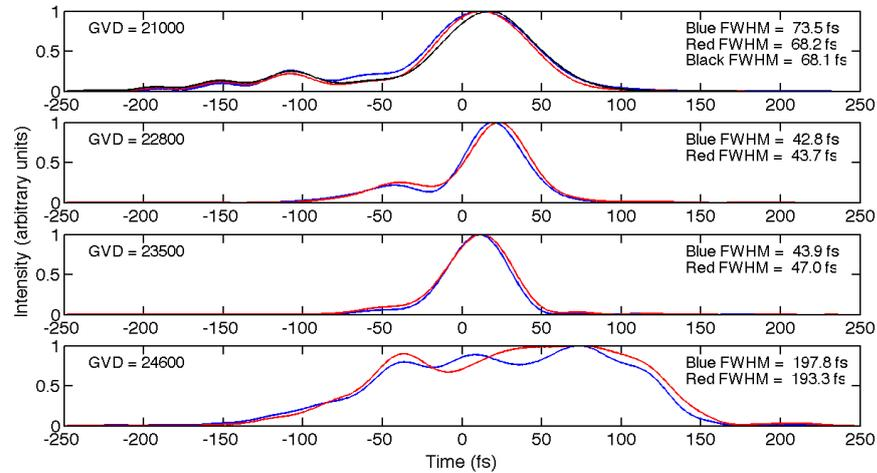
**Figure 7.1.:** The experimentally measured intensity profile of the Astra laser pulse after introducing group velocity dispersions by the dazzler. The red shots and blue shots were taken two hours apart, demonstrating the level of reproducibility of the intensity profiles.
