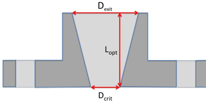
**Figure 6.4.:** The gas jet nozzle design [83] detailing the parameters which characterise the gas jet target. Properties of the gas jet such as density, Mach number and sharpness of the vacuum-gas boundary are set by these parameters.
