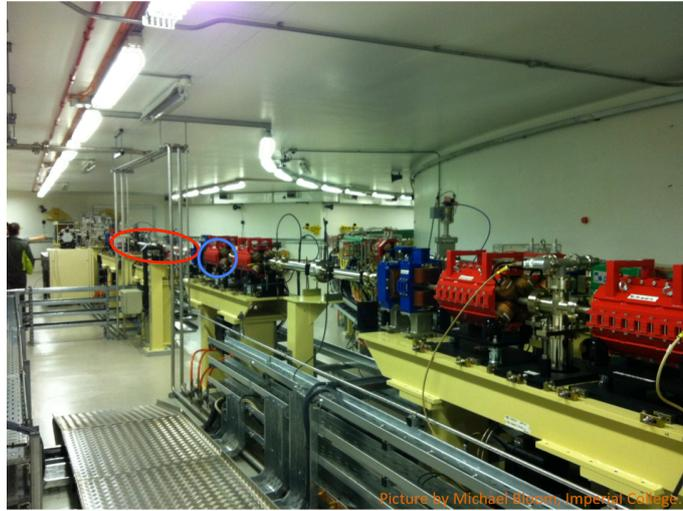
**Figure 4.1.:** The transfer line between the Diamond Light Source’s inner booster ring and outer storage ring (red circle) where the available 6 m of beam line is found. A tuneable quadrupole is positioned before the start of the 6 m of beam line (blue circle) allowing control over the radial size of the Diamond beam. Picture courtesy of Dr. Michael Bloom.
