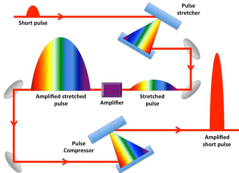
**Figure 6.1.:** Graphic of a short laser pulse undergoing chirped pulse amplification.
