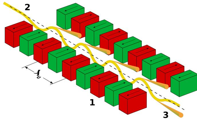
**Figure 1.4.:** A graphic of an undulator [24]. Alternating polarity dipole magnets (1) cause a propagating beam (2) to undulate, radiating bright, coherent synchrotron radiation (3).
