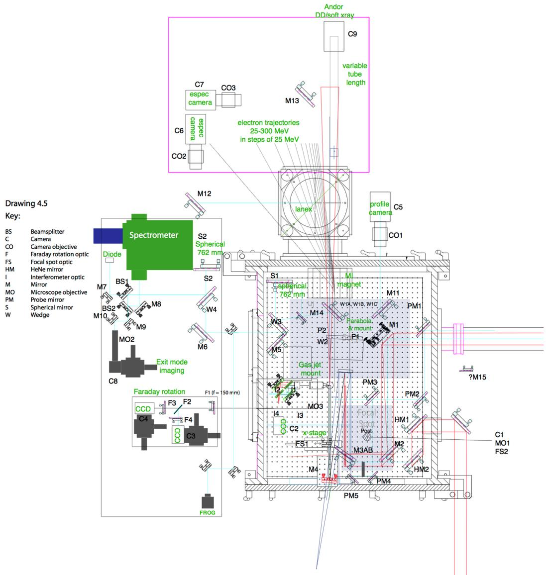
Figure 6.2.: Schematic [77] of the interaction point vacuum chamber (centre), electron spectrometer (above) and imaging diagnostic table (left) for the TA2 experiment.
