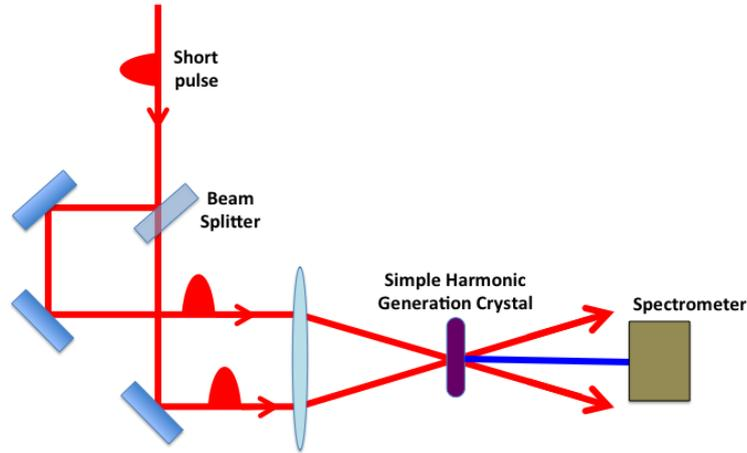
**Figure 6.3.:** Schematic for a frequency resolved optical gating diagnostic. The laser pulse to be measured is split and gated with itself in the non-linear medium, generating a new pulse (blue). The generated pulse is then spectrally resolved with respect to delay.
