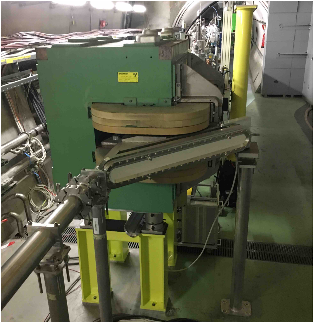
Figure 4.2.: The spectrometer vacuum chamber and dipole magnet installed at AWAKE. The image is taken facing upstream, towards the SPS transfer line. The scintillator (white) may be seen on the exterior surface of the vacuum window at approximately 45^\circ to the beam line.
