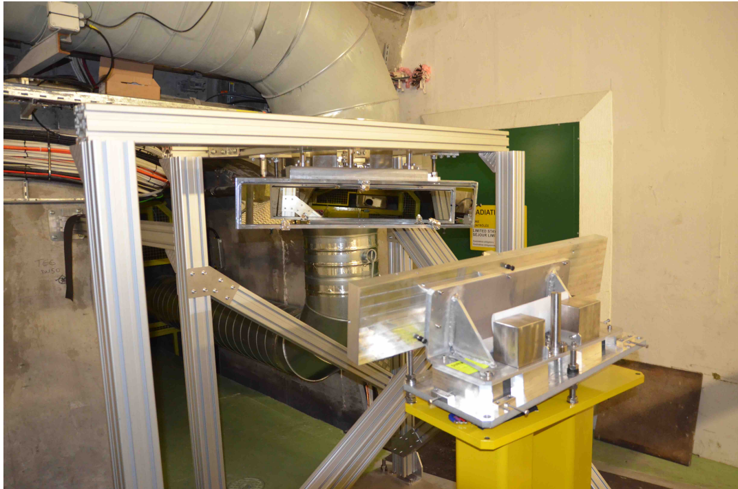
(a) The mounts for M1 and M2 at AWAKE. The camera lens is visible near the centre of M1 (black circle) via its reflection through M2 and M3.
