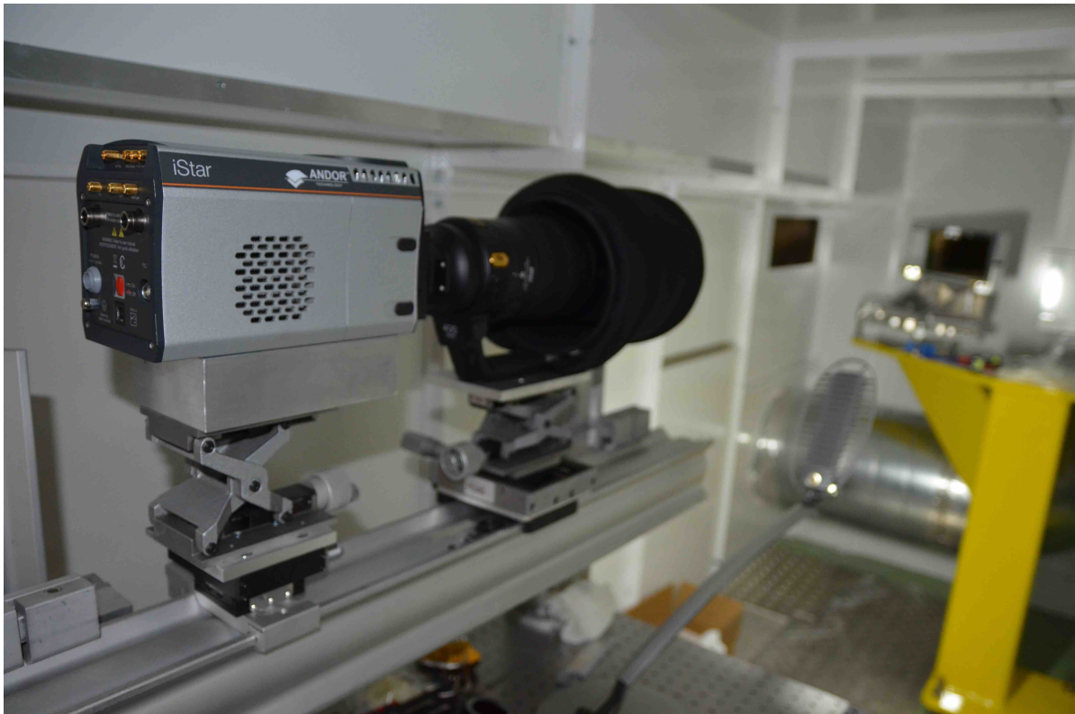
Figure 4.5.: The spectrometer camera and lens in the darkroom. The lens is covered by a lens hood. The final mirror may be seen, out of focus, on the right side of the image.
