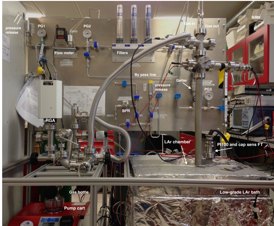
Fig. 3.2: Photo of the LARA gas system and test chamber. Major components are labelled in the figure.
