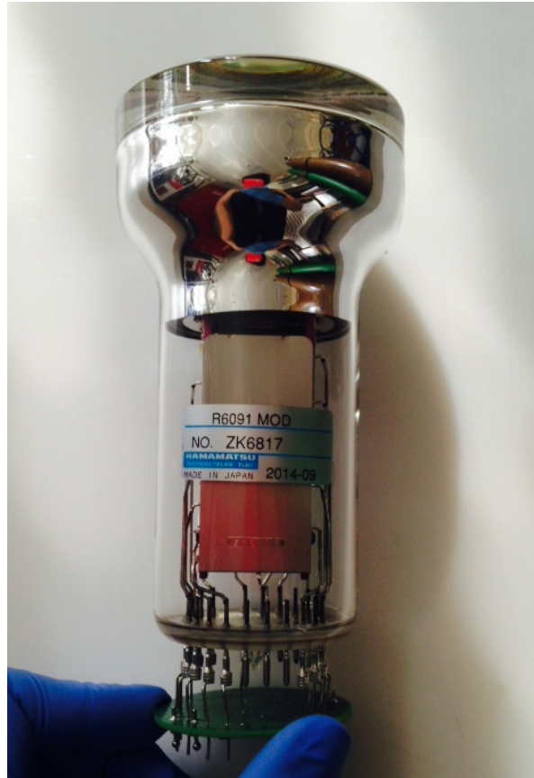
Fig. 3.14: R6091 Hamamatsu photomultiplier tube with in-house made PCB. The platinum underlay below the photocathode makes this PMT suitable to work at cryogenic temperatures.
