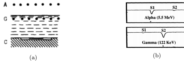
Fig. 1.19: Figure (a) is taken from the original paper of Dolgoshein et al. 1970 in 1970 and corresponds to a three-electrode chamber: A, G, and C represent the anode, grid, and cathode, respectively. An alpha source is placed on the cathode. Figure (b) is taken from the original paper of Suzuki et al. 1993 from 1993. It shows the scintillation signal seen in a xenon two-phase TPC for 5.5 MeV alphas from ^{241}\text{Am} (top) and 122 keV \gamma -rays from ^{60}\text{Co} (bottom).
