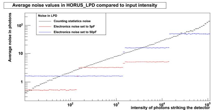
Fig. 4: Average noise values due to counting statistics and electronic noise across the LPD dynamic range.
