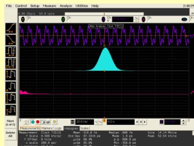
The further tests involved applying filtering on the 3.3 V rail to reduce the jitter readings. In order to do this, LTM4600EV was soldered on a small PCB and this PCB is attached to the CC RTM by cables so that it received the 12V RTM power from the DAMC2. The most promising jitter readings were obtained when a LC filter (1uH/1uF) is attached to the output of the DC/DC converter in addition to the required capacitors.
