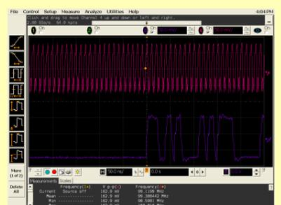
The tests involved using the worst case signal which would cause maximum DC wander on the AC coupled data link. The data is generated such that short bursts of 22-bit Pseudo Random Bit Sequence (PRBS) words are interspersed between long sequences of ones or zeros. The sequence always starts with a predefined start word for synchronisation.
