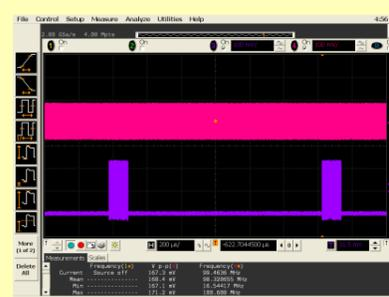
The tests involved using the worst case signal which would cause maximum DC wander on the AC coupled data link. The data is generated such that short bursts of 22-bit Pseudo Random Bit Sequence (PRBS) words are interspersed between long sequences of ones or zeros. The sequence always starts with a predefined start word for synchronisation.
