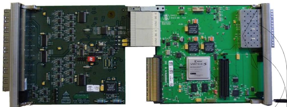
The MTCA.4 AMC board (DAMC2) is designed by DESY as a multi-purpose FPGA hardware platform for various projects in DESY and provides the processing capability for the CC functionality.
