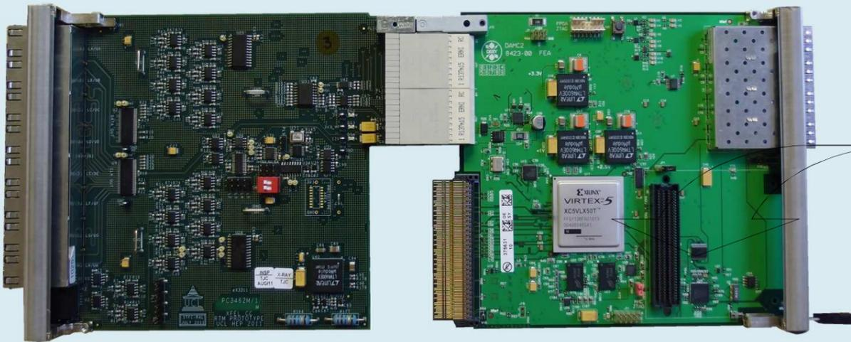
The MTCA.4 AMC board (DAMC2) is designed by DESY as a multi-purpose FPGA hardware platform for various projects in DESY and provides the processing capability for the CC functionality.
