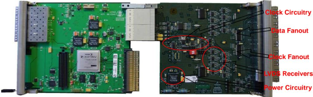
The CC system is responsible for the synchronisation of the detectors and the DAQ system to the general EuXFEL timing. The EuXFEL facility will generate coherent and intense X-ray flashes with a  $\sim 4.5$  MHz bunch frequency. The Timing Receiver (TR) board housed in the same crate as the CC system delivers the bunch clock to the CC through the MTCA.4 backplane.
