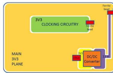
We envisage further improvements when this filtering scheme is employed on the final version of the CC RTM and the voltage plane for the clocking circuitry is separated from the main power plane by a ferrite bead.
