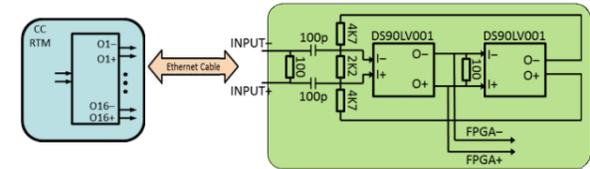
The clock and the data links to the FEE units are AC all coupled. Because the data sent to the FEEs is not DC balanced, a special circuitry on the receiver side is used to alleviate the DC wander. This circuitry limits the maximum cable length to be used for the FAST data link.
