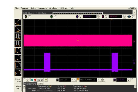
The tests involved using the worst case signal which would cause maximum DC wander on the AC coupled data link. The data is generated such that short bursts of 22-bit Pseudo Random Bit Sequence (PRBS) words are interspersed between long sequences ones or zeros. The sequence always starts with a predefined start word for synchronisation.
