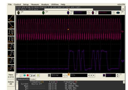
The tests were performed using Ethernet cables of lengths 10m, 15m, 20m, 30m and 50m. There were no errors observed during a period of more than 24 hours with the CAT6 SFTP cables up to 30m. If there is a need to support a 50m cable length MLVDS drivers are going to be tested for data and clock transmission.
