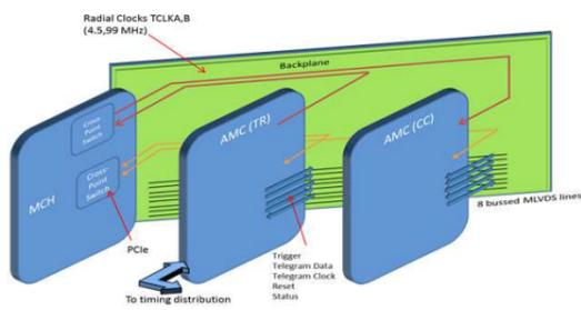
The link between a FEE unit and the CC system consists of 3 LVDS pairs to transfer the 99 MHz clock, FAST data and the VETO information and 1 pair to receive the status information from the unit. One CC RTM can support up to 16 FEE units which in turn support a 1 mega pixel detector.
