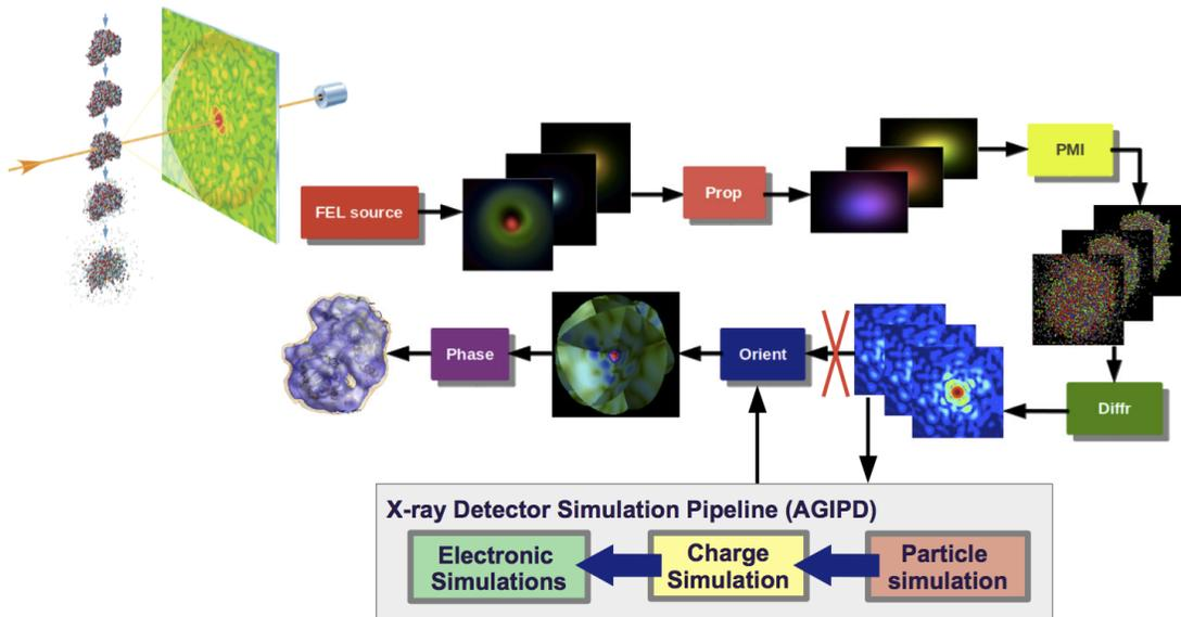
**Figure 3:** Overview of *simS2E* simulation pipeline and where *XDSP*'s hook into the simulation, providing an realistic estimate of detector performance.
