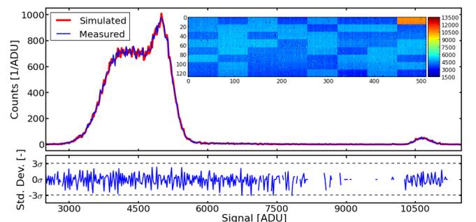
**Figure 2:** Comparison of spectra of simulated and measured dark images from an AGIPD prototype module. Residuals in terms of  $1\sigma$  experimental uncertainties are shown. Inset: single simulated image.
