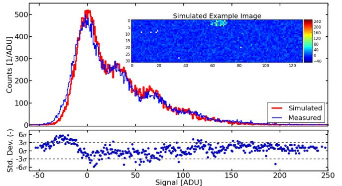
**Figure 1:** Comparison of spectra of simulated and measured pencil beam images from a LPD prototype tile. Residuals in terms of  $1\sigma$  experimental uncertainties are shown. Inset: single simulated image after offset and common-mode corrections.
