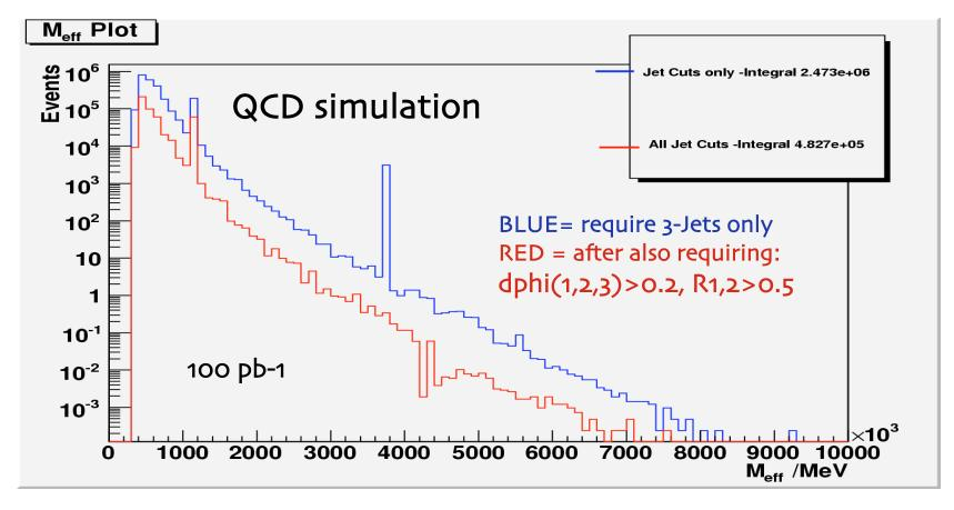
Imposing cuts on dphi and R1,2 removes > 80% of QCD background (according to this MC simulation!) - can suppress further by cuts on e.g. MET
