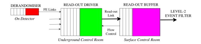
RODs and ROBs contain buffers which can be full, necessiting dead-time introduction
