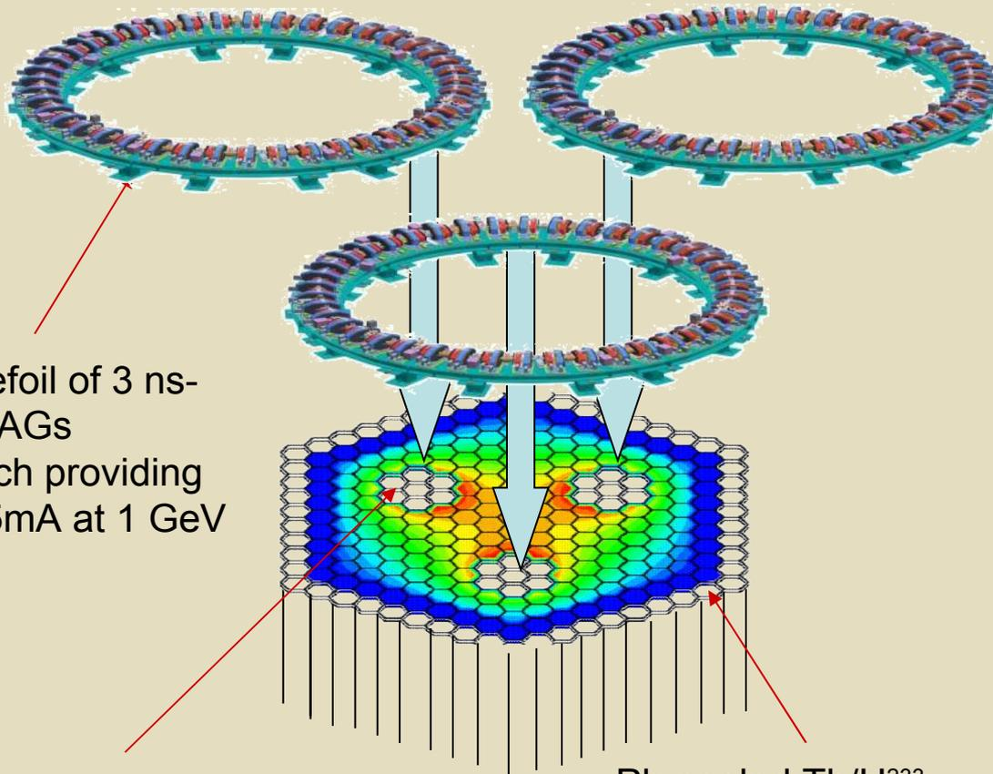
Trefoil of 3 ns-FFAGs each providing 3.5mA at 1 GeV
