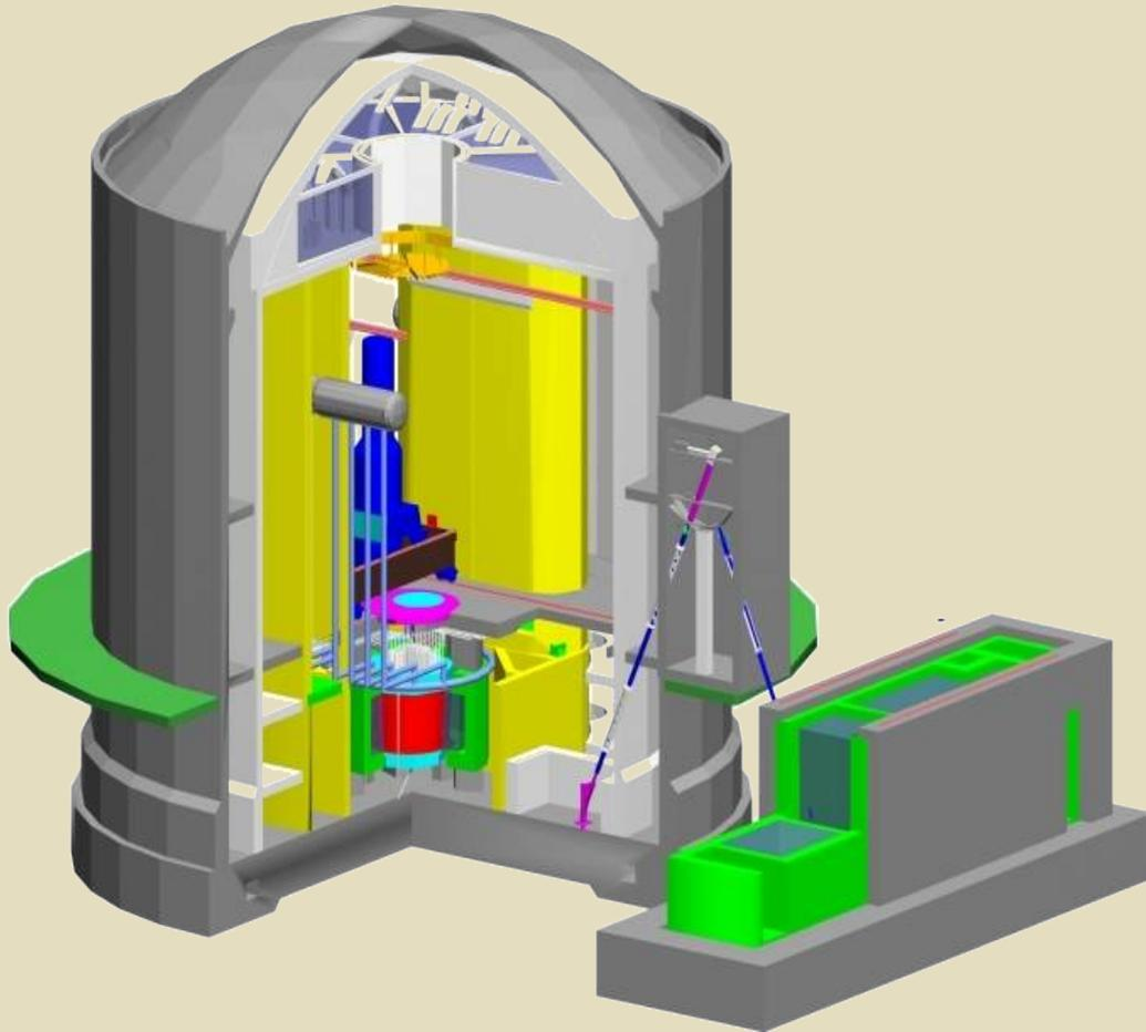
The planned AHWR (India) is a vertical pressure tube type, boiling light water cooled and heavy water moderated reactor using  $^{233}\text{U}$ -Th MOX (Mixed Oxide) and Pu-Th MOX fuel.
