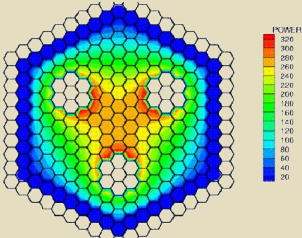
Power density distribution (W:cm<sup>3</sup>) in a lead-cooled ADSR with Th:U<sup>233</sup> fuel.
