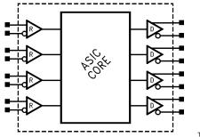
FIGURE 11. ASIC Cell Implementation of LVDS
