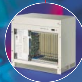
The aluminum/sheet steel design of the COMPACT-I system balances performance and economy for medium/high volume applications.
