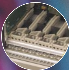
UL recognized ground connections allow a pluggable earth/ground contact for rear CPCI I/O modules.
