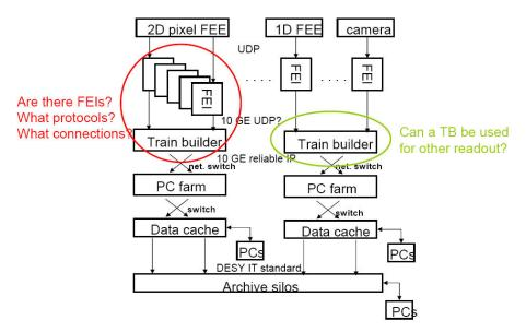
, where the 2D detector FEIs (Front End Interfaces) have been drawn but in reality are part of the front end systems of the detectors, they are not part of the TB. The idea of using the TB in the non 2D pixel detectors should not be forgotten, but it is unlikely due to the very much smaller train data volumes,  $\leq$  1%, originating from these detectors. The DAQ requirements of these detectors should be satisfied using a FEI to buffer data and send it by TCP to the PC farm layer.
