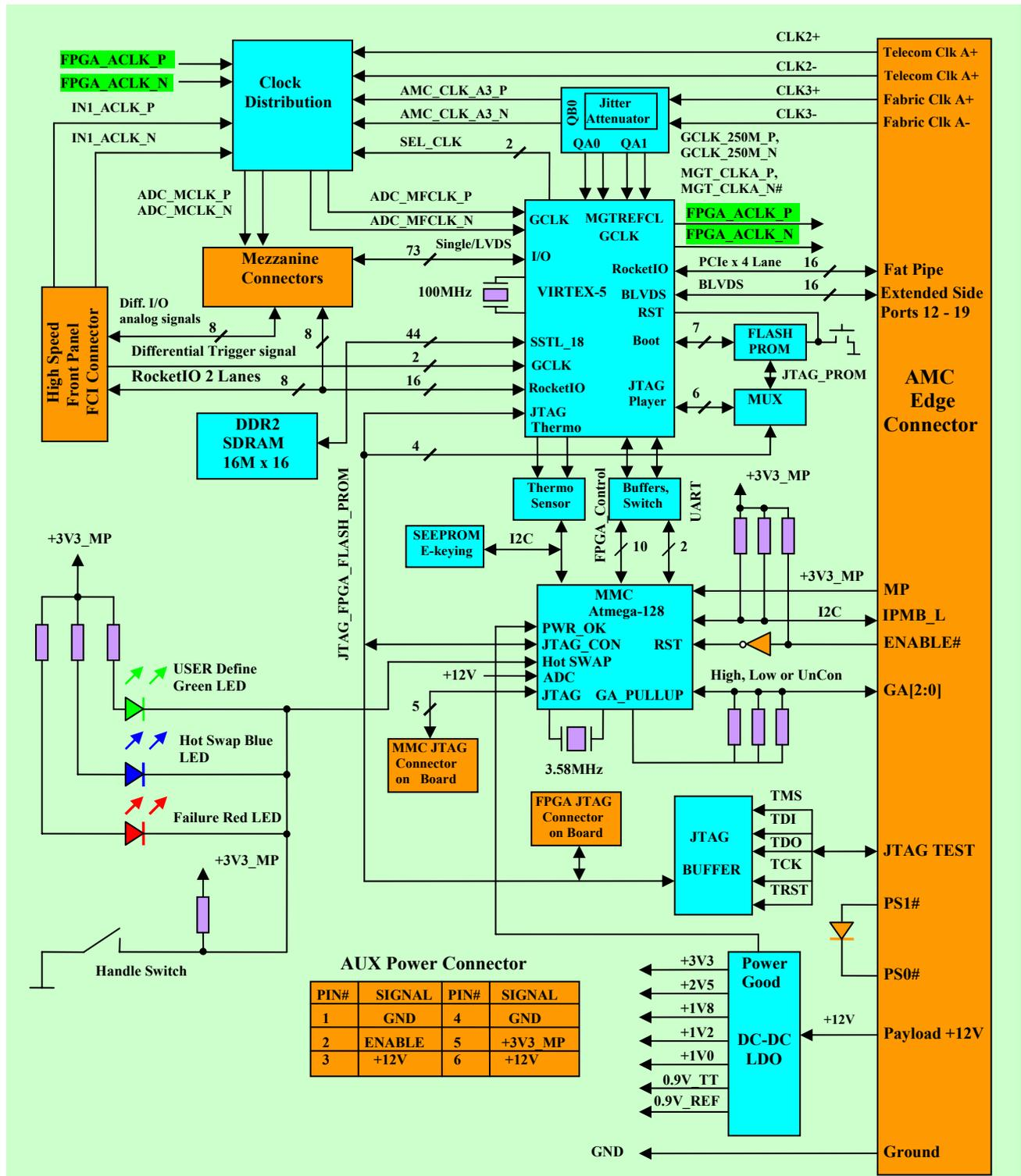
Figure 2 Block diagram of AMC-01
