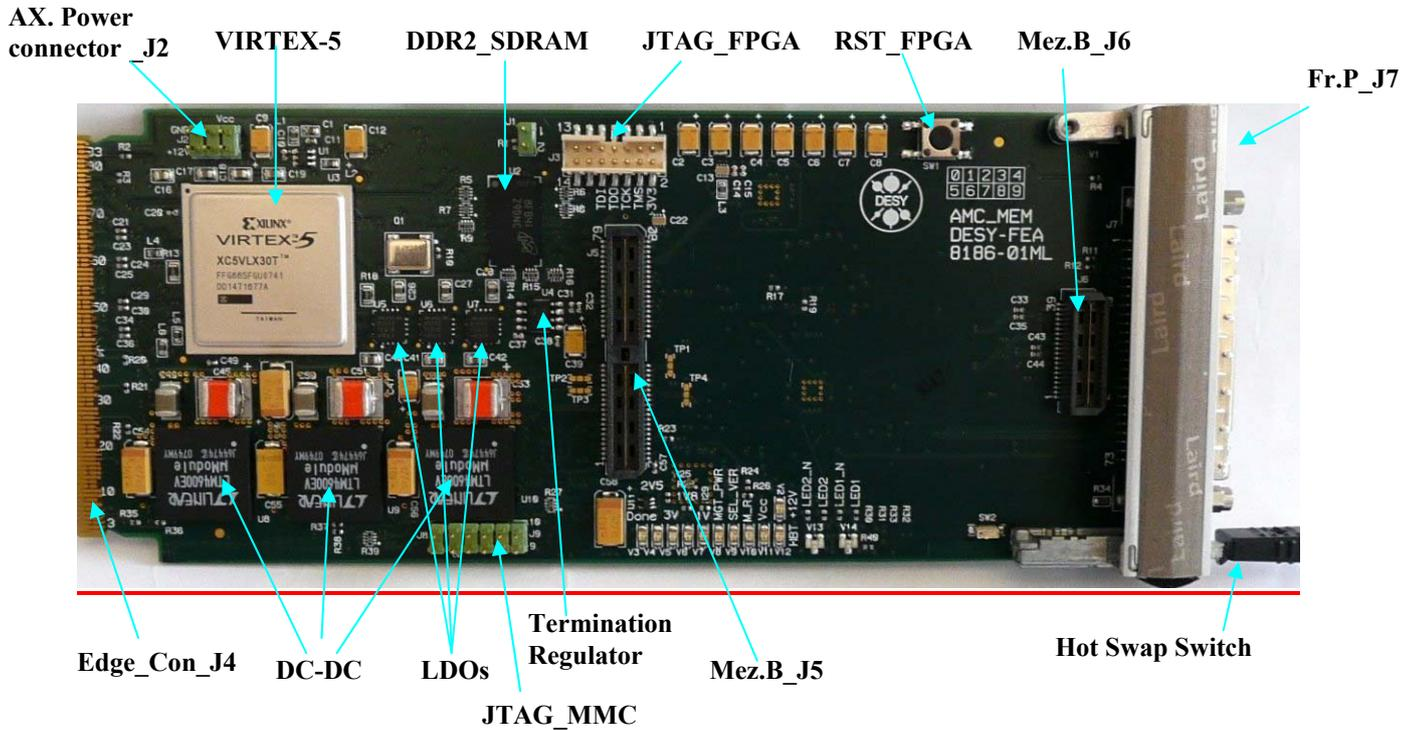
Figure 1 AMC-01 top view
