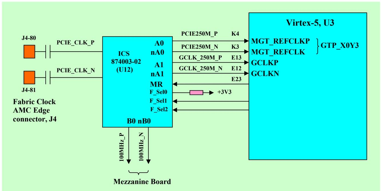
Figure 5 PCI Express clocking and control
