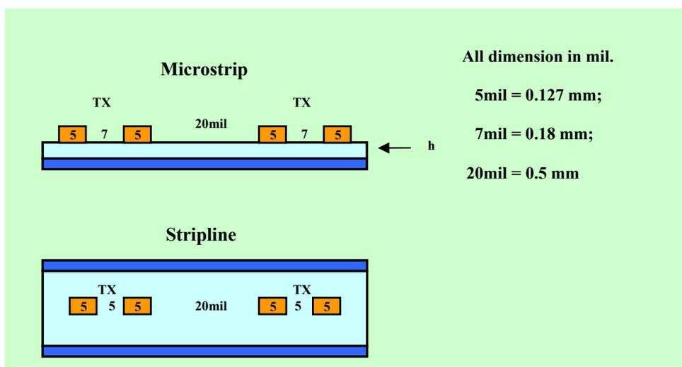
Figure 21 Trace width and spacing
