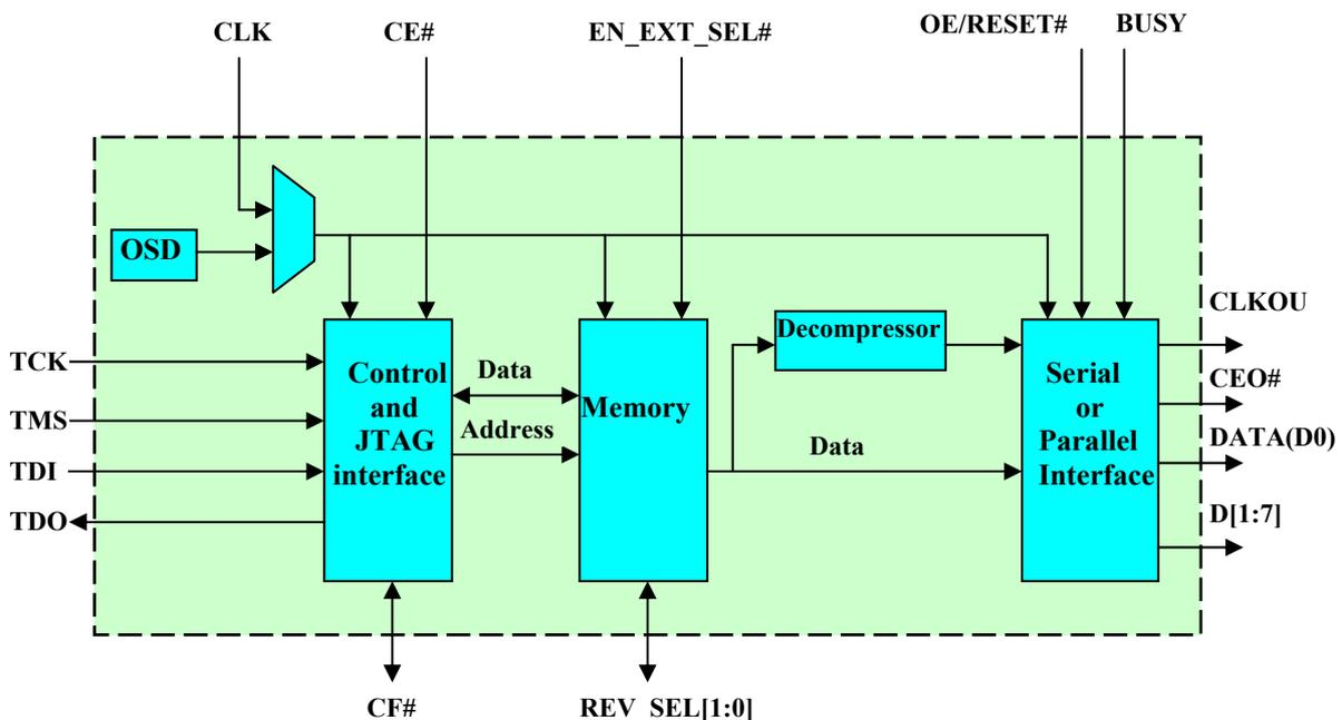
Figure 13 XCFxxP Platform Flash PROM Block Diagram
