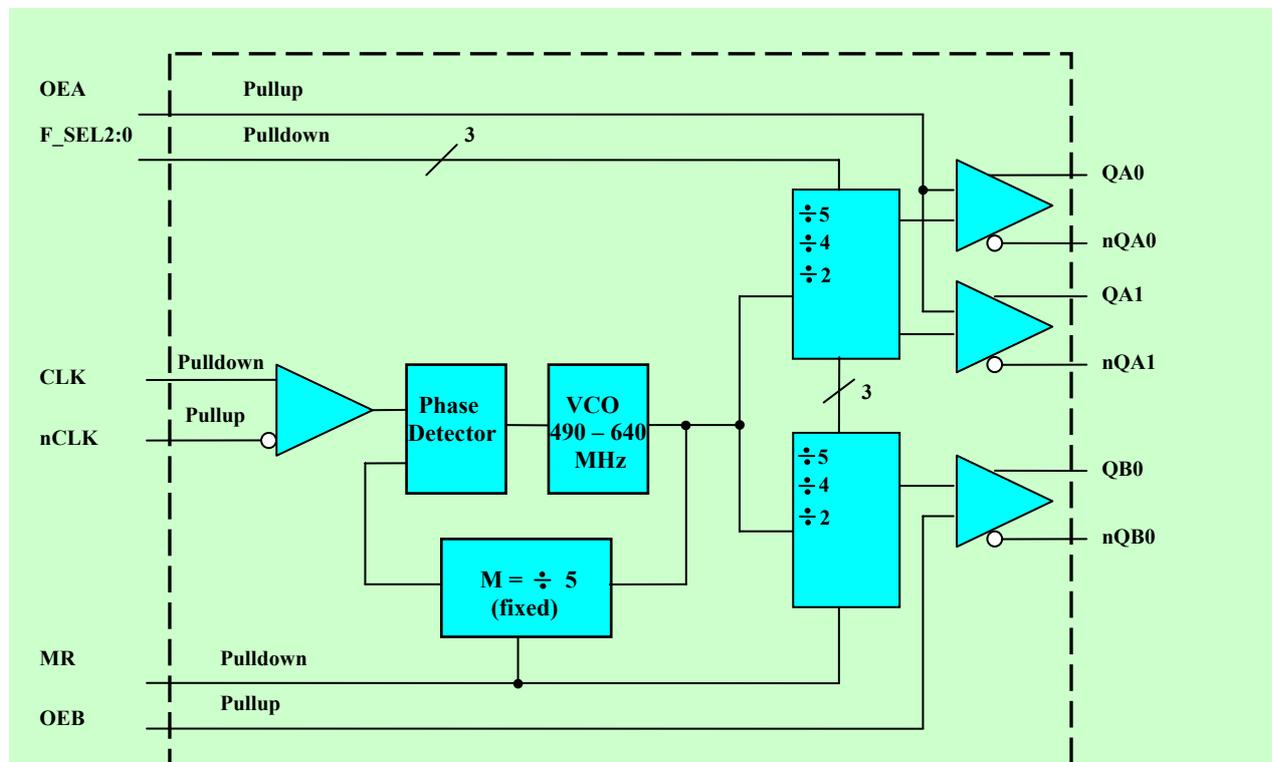
Figure 6 Block diagram ICS874003-01
