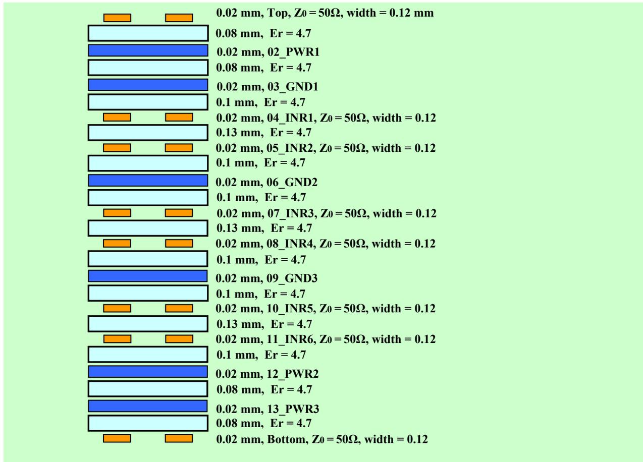
Figure 20 AMC-01 PCB Stack-up
