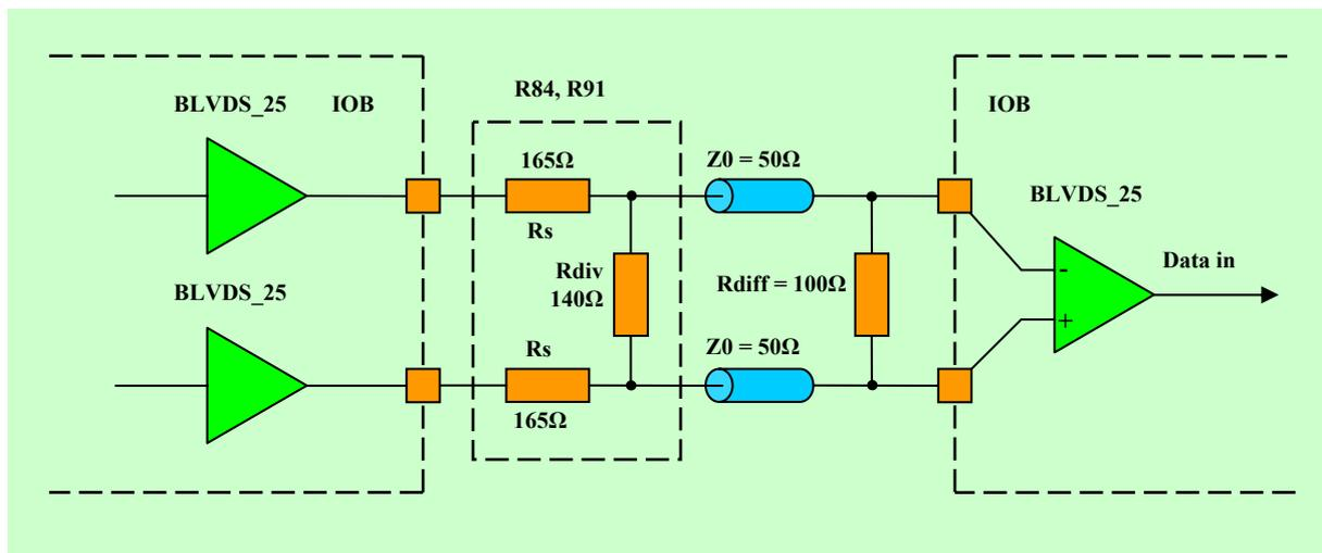
Figure 10 BLVDS Transmitter Termination
