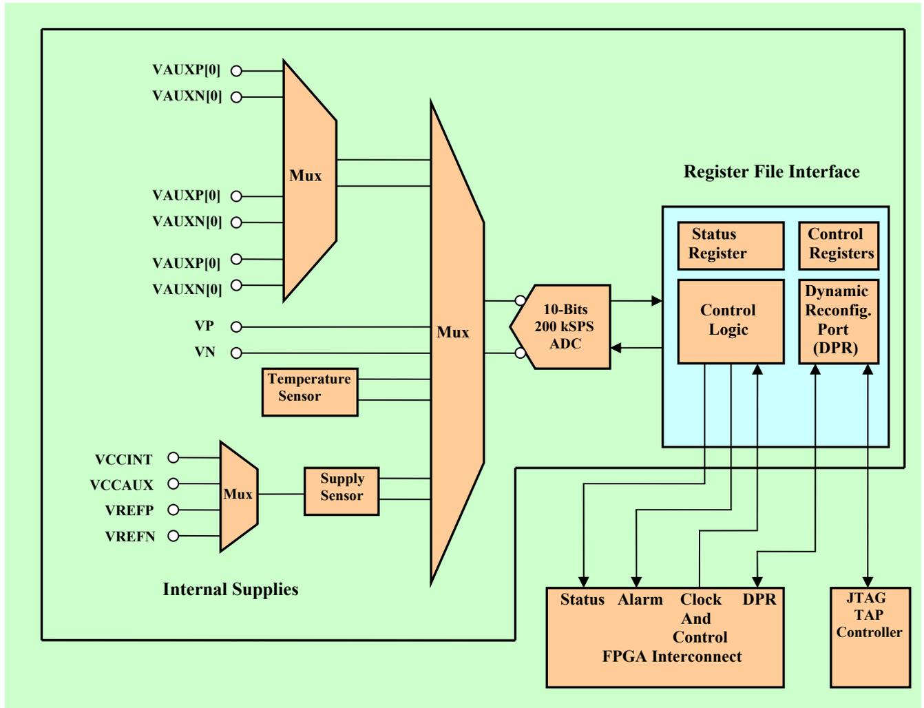
Figure 3 Block diagram of System Monitor
