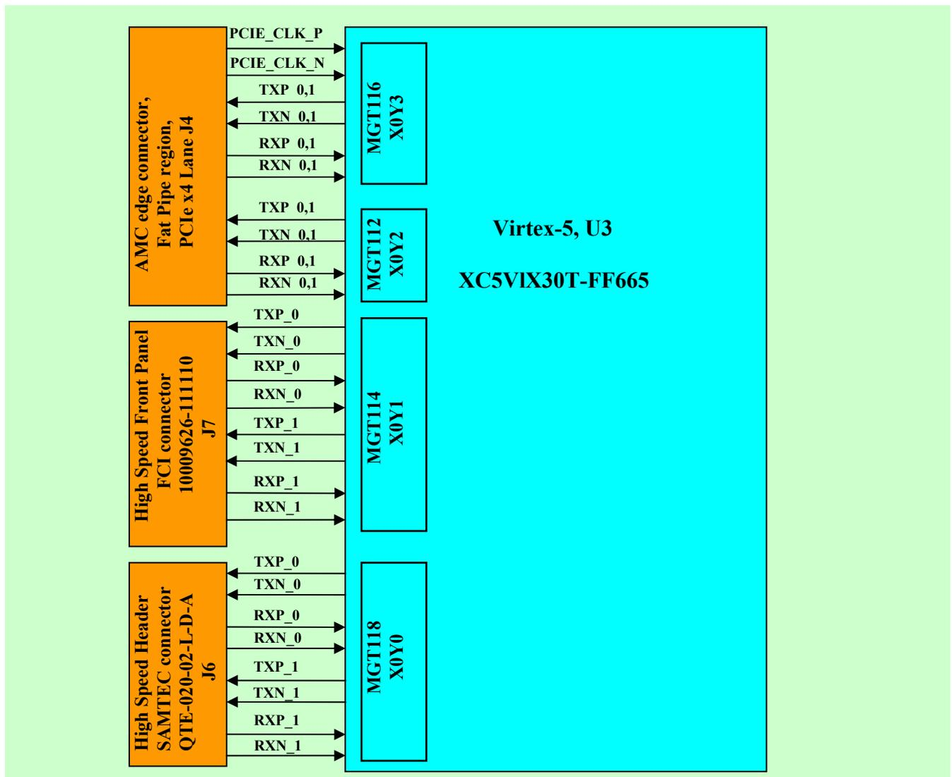
**Figure 4 GTP ports of AMC-00**
