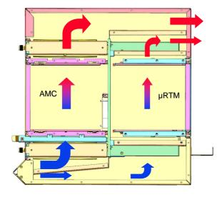
The air intake is at the front bottom side of the chassis, the air exhaust is the rear upper side. Air baffles separate the air flow for the front card section and the rear card section in order to maximize cooling capability.
