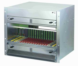
Front slots conform to MicroTCA specification PICMG MicroTCA.0 R1.0
