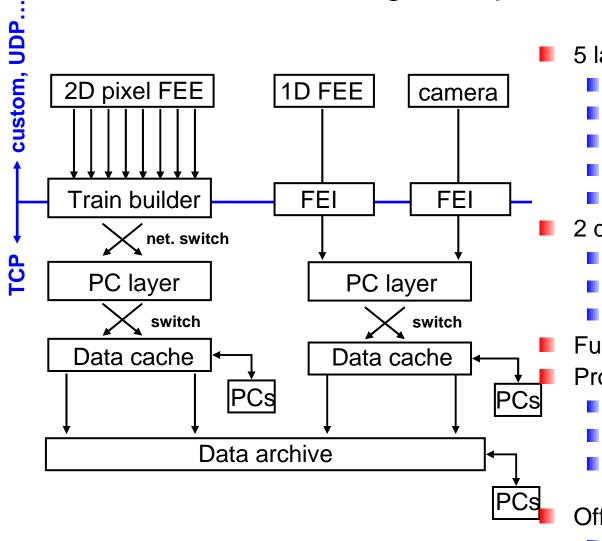
5 layers Front End Electronics FEE Front End Interface FEI PC layer Data cache (temporary) Data archive (permanent) 2 data protocols FEE to FEI = custom, UDP,... FEI to data archive = TCPProtocol conversion at FEI/TB Full bandwidth into cache Processing TB (train building+reduction?) PC layer (algo+rejection) Data cache (algo+rejection using expt. downtime) Offline processing/access Data archive
