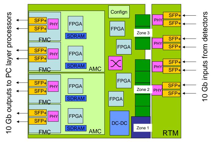
Double width AMCs and FPGA mezzanine FMCs ease prototyping/development
