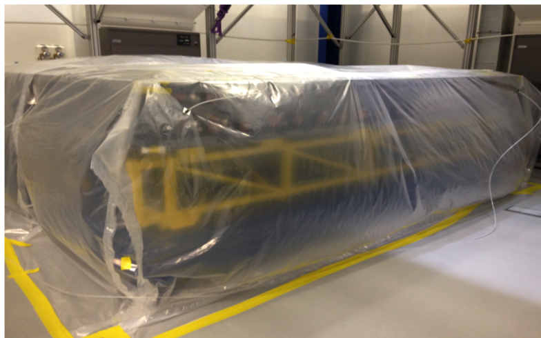
Figure 7.11: Photograph of the anti-radon tent covering the C-section.
