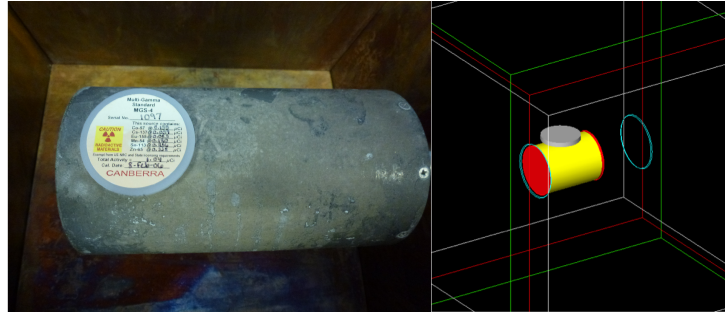
Figure 8.6: (Left) The MGS on the detector endcap for measurement. (Right) Simulated MGS on detector endcap at the same location in order to determine detection efficiency.
