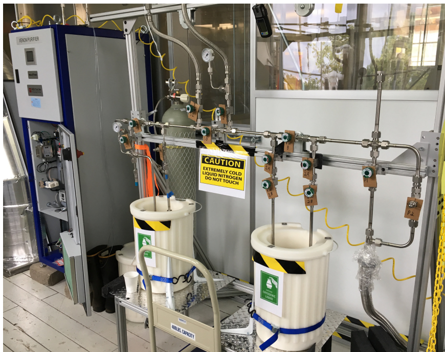
Figure 4.19: A pictorial diagram of the portable radon harvesting system used at the SAL for the getter radon emanation measurement. The emanated radon is collected by transferring through one of the traps held under LN_2 temperature. The trap is later transported to a radon emanation facility for counting.
