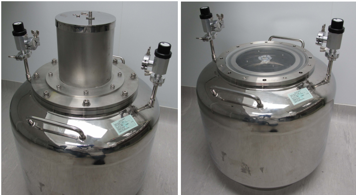
Figure 4.2: Pictorial diagram of the electrostatic detector used for the radon emanation results published in this work. Left shows the detector in full operational mode and the right shows it without its lid, where the feedthrough for the PIN-diode can be seen.
