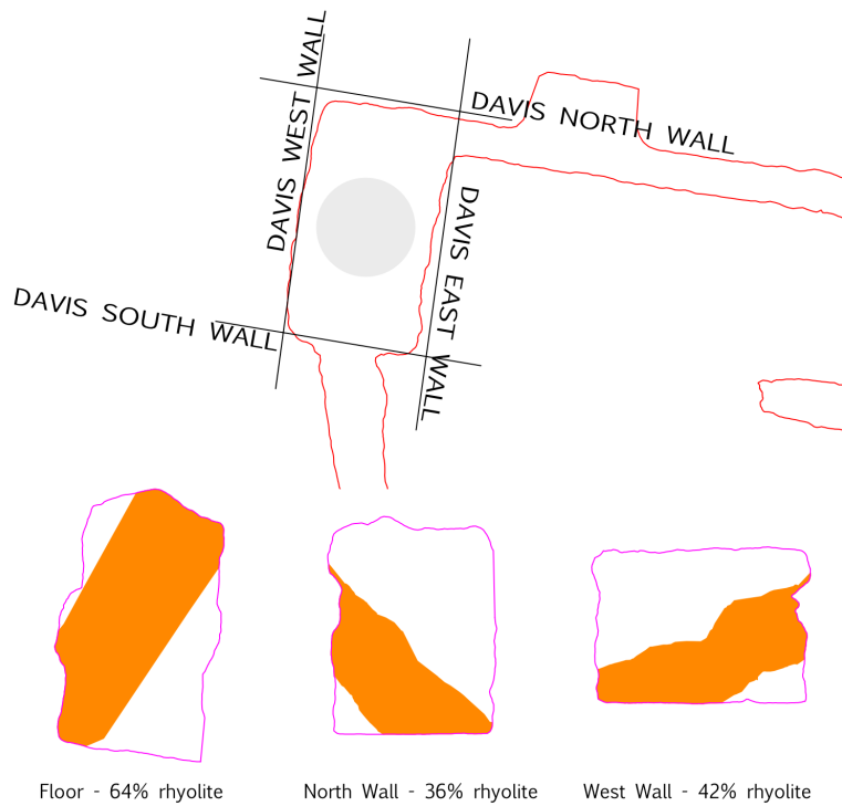
Figure 3.3: Diagram of the Davis cavern highlighting the naming conventions of the wall locations and the rhyolite intrusion layers in orange with the estimated percentage coverage of rhyolite. The water tank is marked with a grey circle. The ceiling is estimated at 0% rhyolite, the south wall at 5% and the east at 2% [133]. Diagram adapted from [2].
