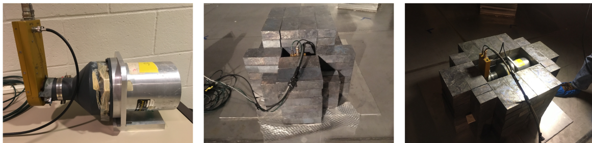
Figure 3.4: A photograph of the 5-inch NaI(Tl) detector (left), showing the pre-amplifier, PMT and NaI crystal. The right two images are showing the lead shielding configuration in measuring \gamma -rays from the bottom (centre) and from above (right).
