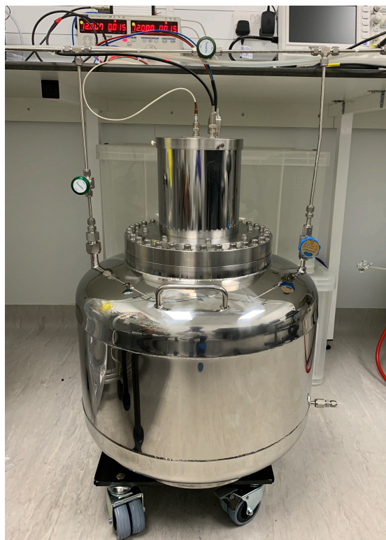
Figure 7.3: Pictorial diagram of the 80 L high-sensitivity PIN-diode radon detector.
