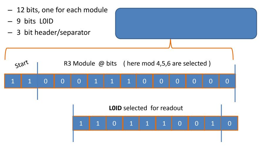
Total = 24 bit times @ 80MHz,  $\rightarrow$  300ns per R3 packet Allows a stave to have a maximum R3 rate of 3.3MHz
